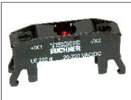
Status Indicators in RED colour are available for multiple limit switches with 12 mm plunger spacing and switching element ES502E with an operating voltage of 20-230 V AC/DC. An electronic control ensures the same luminous power is retained, irrespective of the voltage applied.
