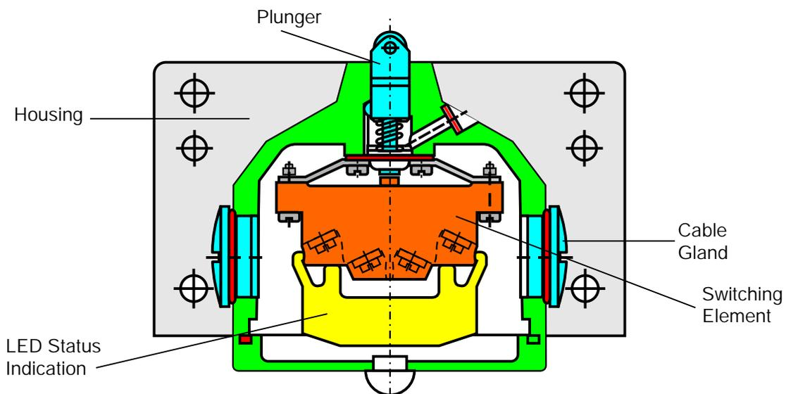
The system drawing shows in clear detail, the perfected design features of the TEKNIC EUCHNER precision limit switch. The material used by TEKNIC EUCHNER for the enclosure is a special aluminium alloy. The enclosure surface and thus the plunger guide are transformed by a special surface coating into an aluminium oxide layer. This surface, combined with the hardened & polished plunger, offers particularly high wear and corrosion resistance.
